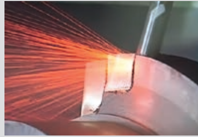
Ceramic milling cutters in use: Blisk machining (plunging), Inconel
