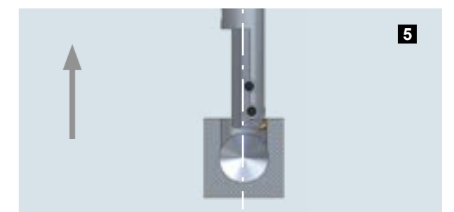
Spindle ON. Execute deburring in working feed backwards.
