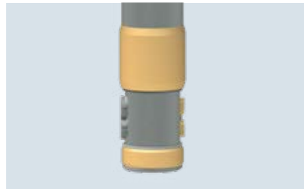
Image 3: SOLO with retracted blade protected by a guide bushing ahead and one after the blade.
