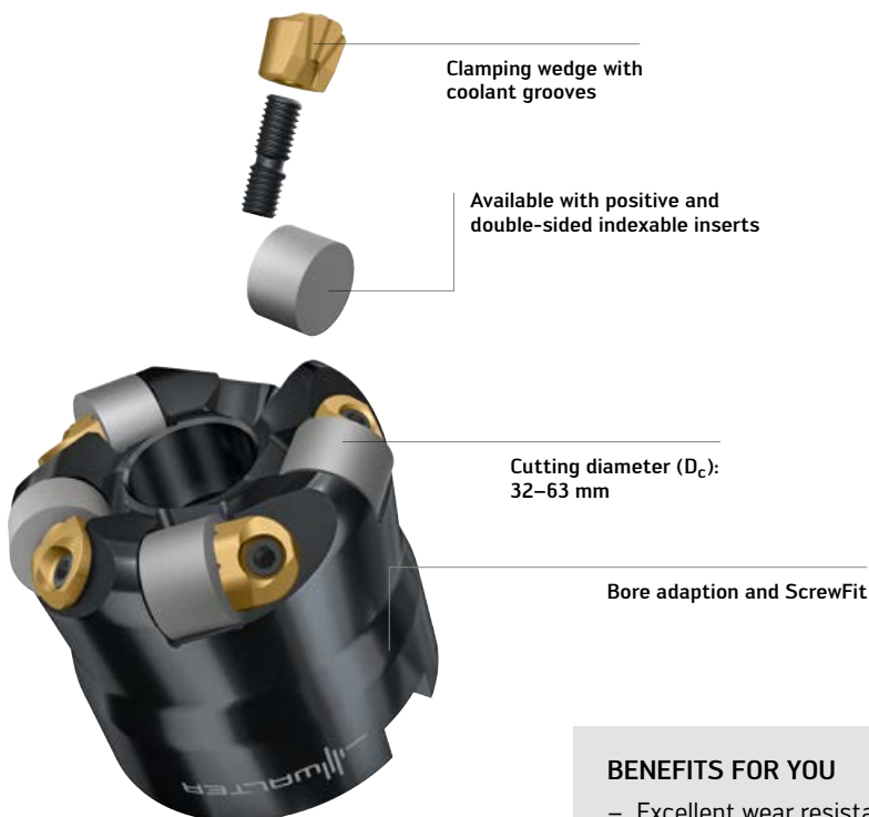
New button insert milling cutter with ceramic inserts
